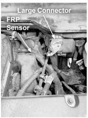
*pliers*). Once released, press in directly on the lock tab as you pull to release the connector. Connect both connectors to the EZX harness.
